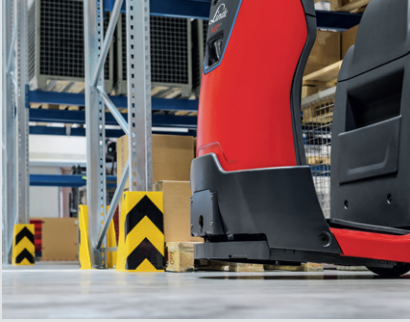
Linde BlueSpot™ and bumper including safety scanner
